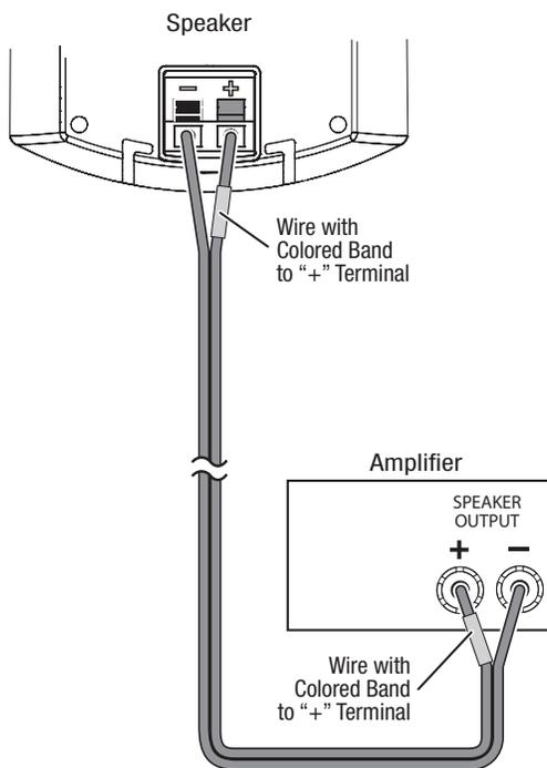
Connect the speakers to the proper amplifier channels:
