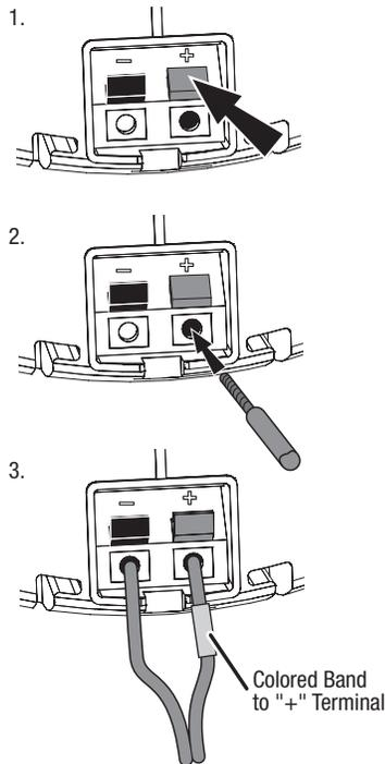
Connect the speaker's "+" terminal to the amplifier's "+" terminal:
